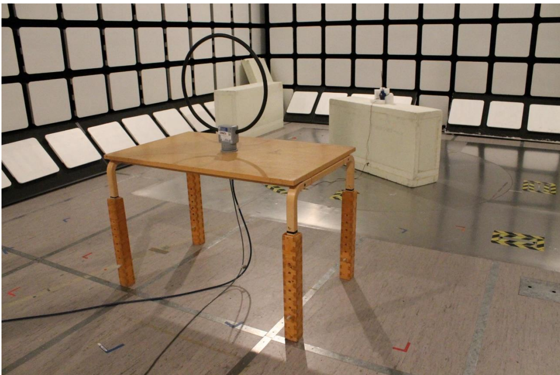
Photograph 2. Radiated Spurious Emissions 9 kHz – 30 MHz
