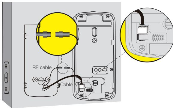
**C** Keep the thumb turn in vertical position, push the cable and RF cable back to the hole of the mounting plate and install the interior assembly.
