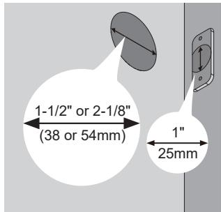
Measure to confirm that the hole in the door edge is 1" (25mm).
