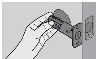
Hold the latch in front of the door hole, with the latch face flush against the door edge. Is the slotted hole centered in the door hole?
