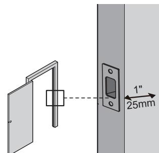
**Notes:** Make sure the door frame is aligned with the door.
