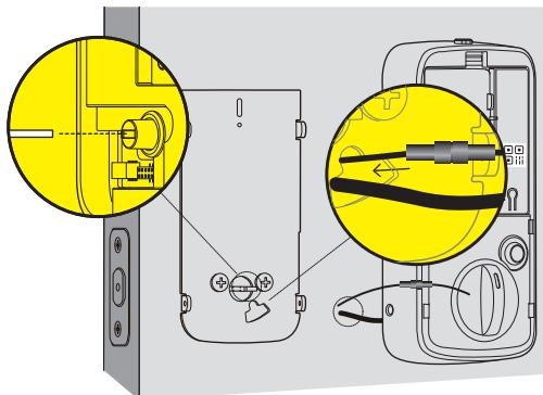
**D** Secure the interior assembly with 3 screws.
