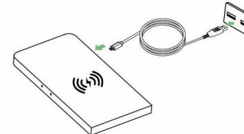
3. If a receiver coil of a charging device is misaligned from the center of the product, it may not be properly charged.
