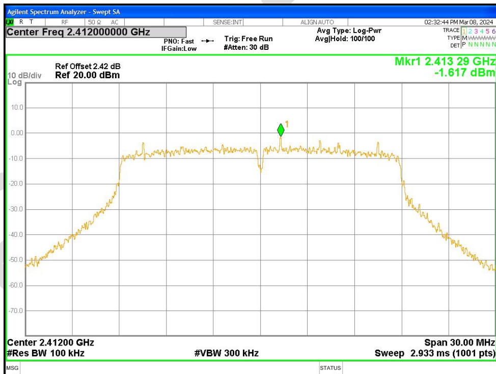
Band Edge NVNT n20 2412MHz Ant2 Emission
