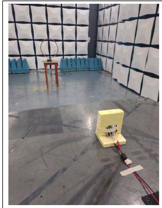
**900 MHz Radio, Radiated Spurious Emission: 30 MHz to 1000 MHz**
