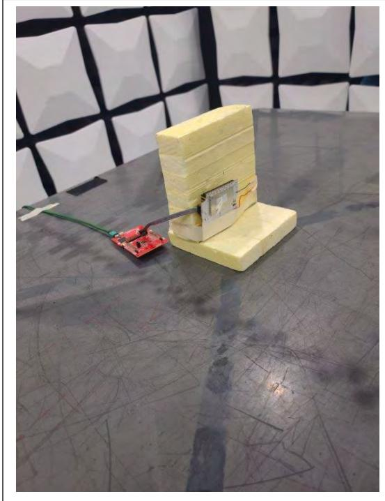
**BLE, Radio Setup: Greater Than 1 GHz**
