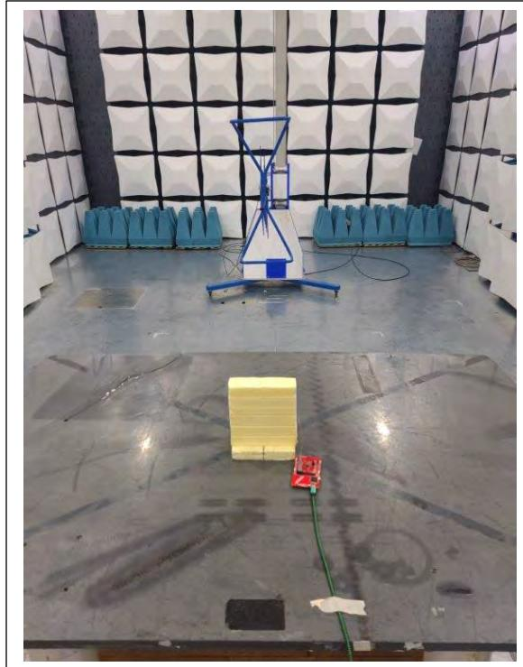
**BLE, Radiated Spurious Emissions: Greater Than 1 GHz**
