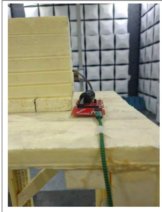
**BLE, Radiated Spurious Emissions: 0.009 MHz to 30 MHz**
