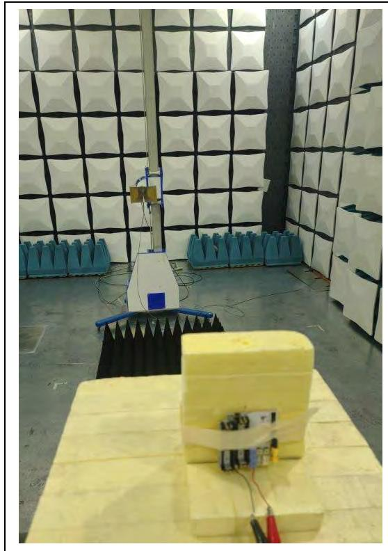
**900 MHz Radio, Conducted Output Power, Occupied Bandwidth, and Conducted Spurious Emissions**
