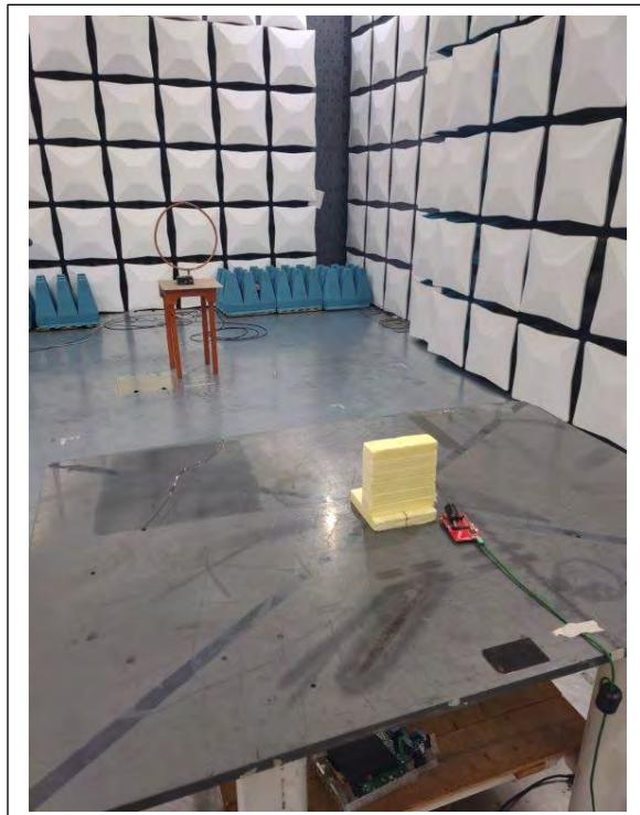
**BLE, Radiated Spurious Emissions: 30 MHz to 1000 MHz**
