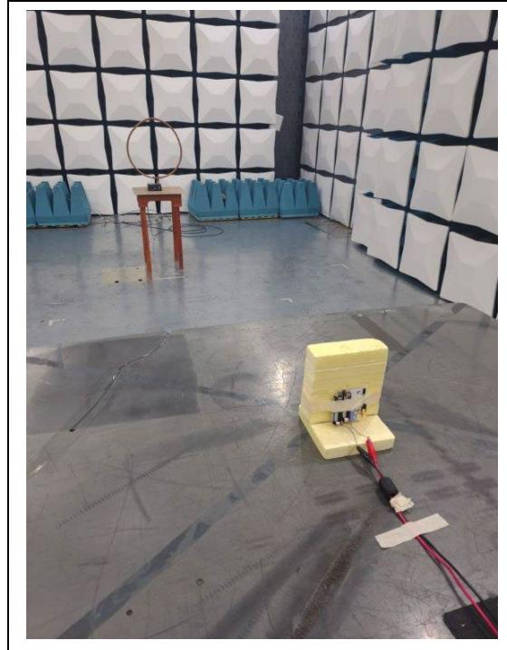
**Radiated Spurious Emission: 30 MHz to 1000 MHz**
