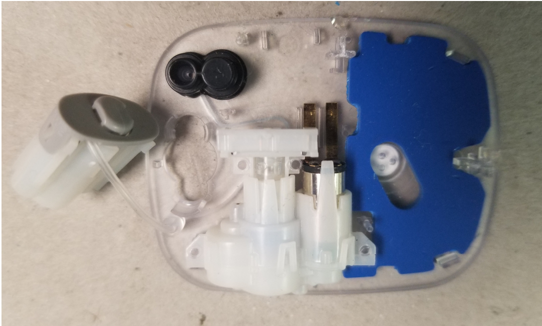
Figure 3: Integrated subassembly without PCBA (grey Insertion Mechanism, Baseplate, Pump and Motor)
