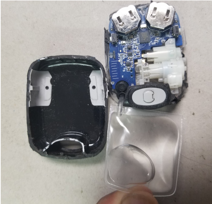
Figure 2: TOP enclosure, Integrated subassembly and reservoir bag
