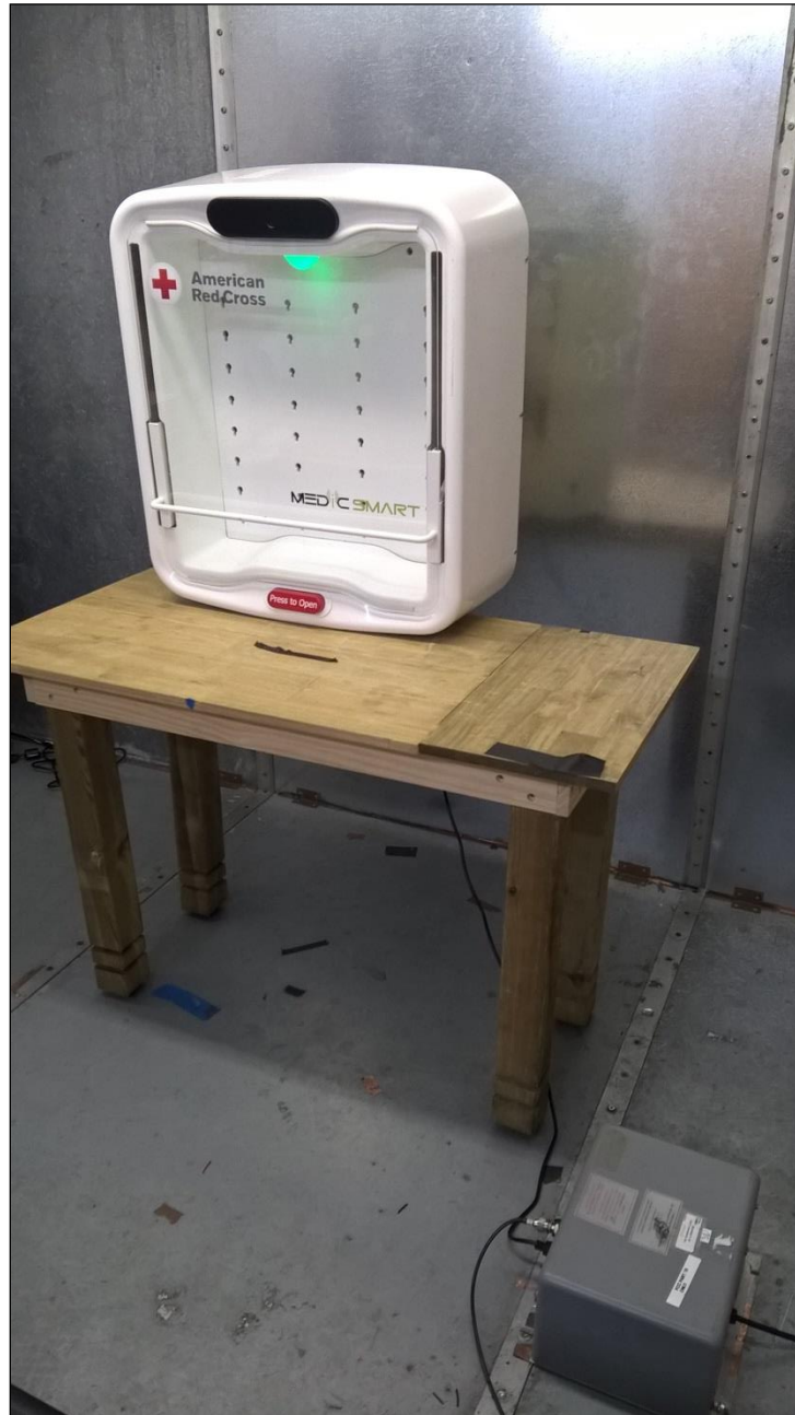
Photograph 1. Conducted Emissions, 15.207(a), Test Setup
