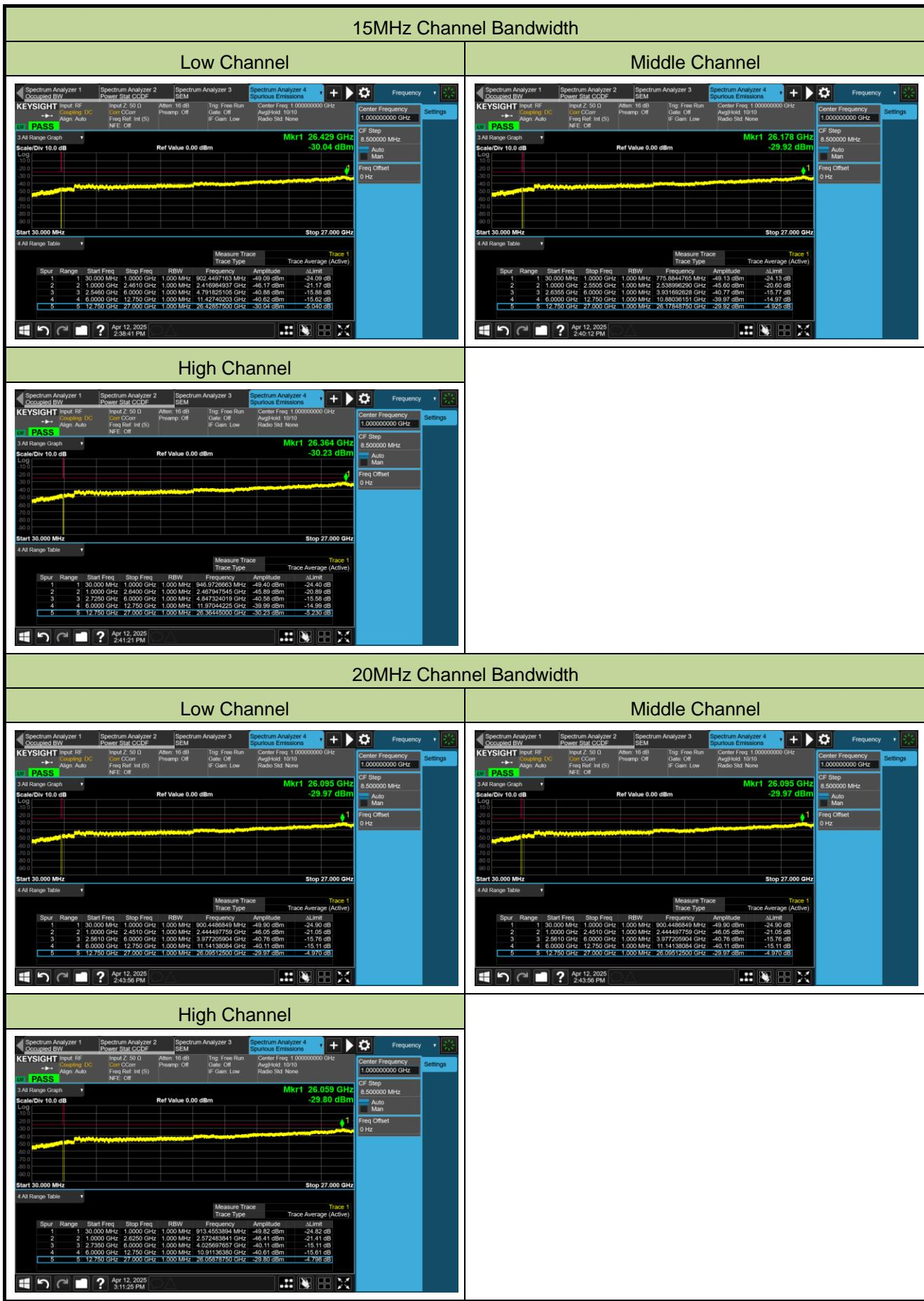
**A.7 Radiated Spurious Emissions Test Result**
