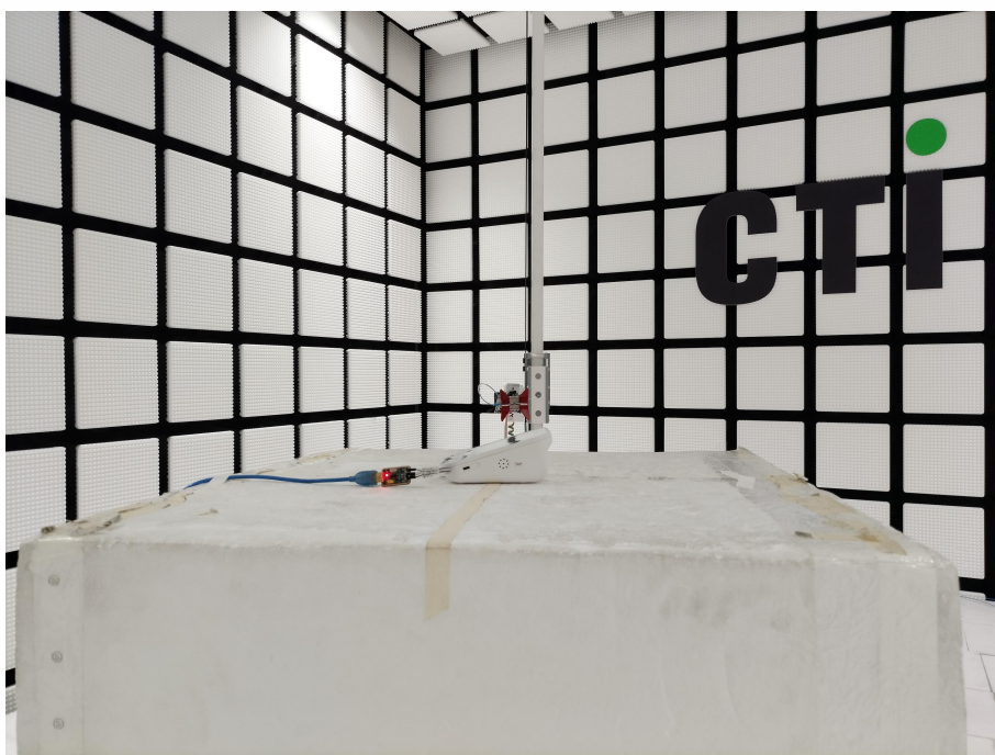
Radiated spurious emission Test Setup-2(Above 1GHz)
