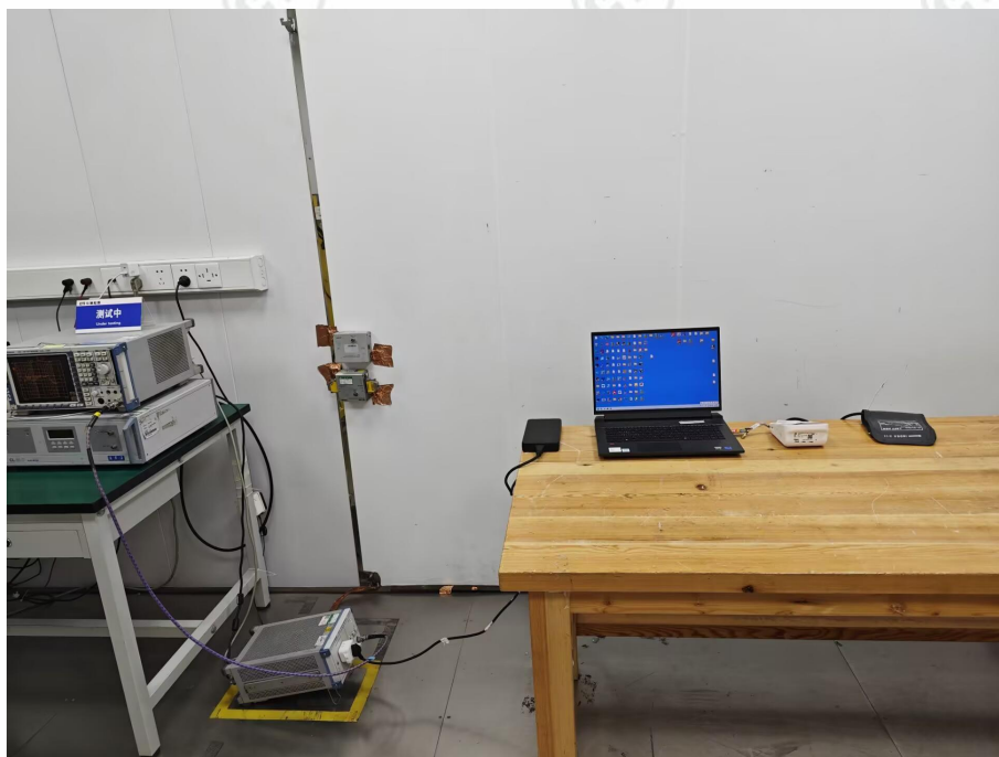
Conducted Emissions Test Setup
