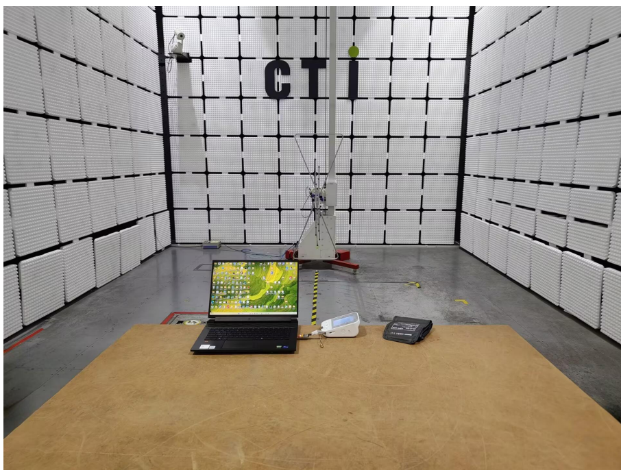
Radiated spurious emission Test Setup-1(Below 1GHz)
