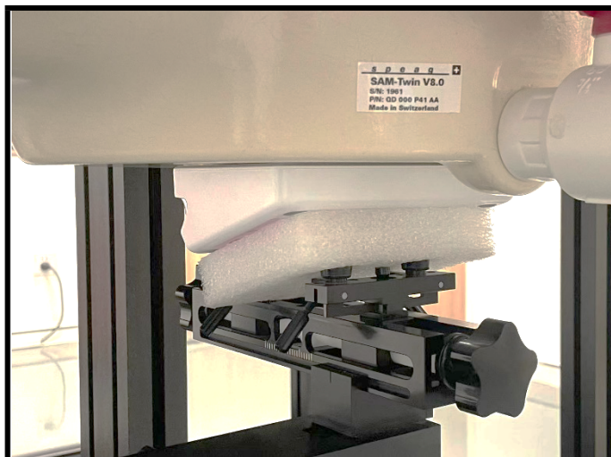
Front Face of EUT with 0 cm Gap
