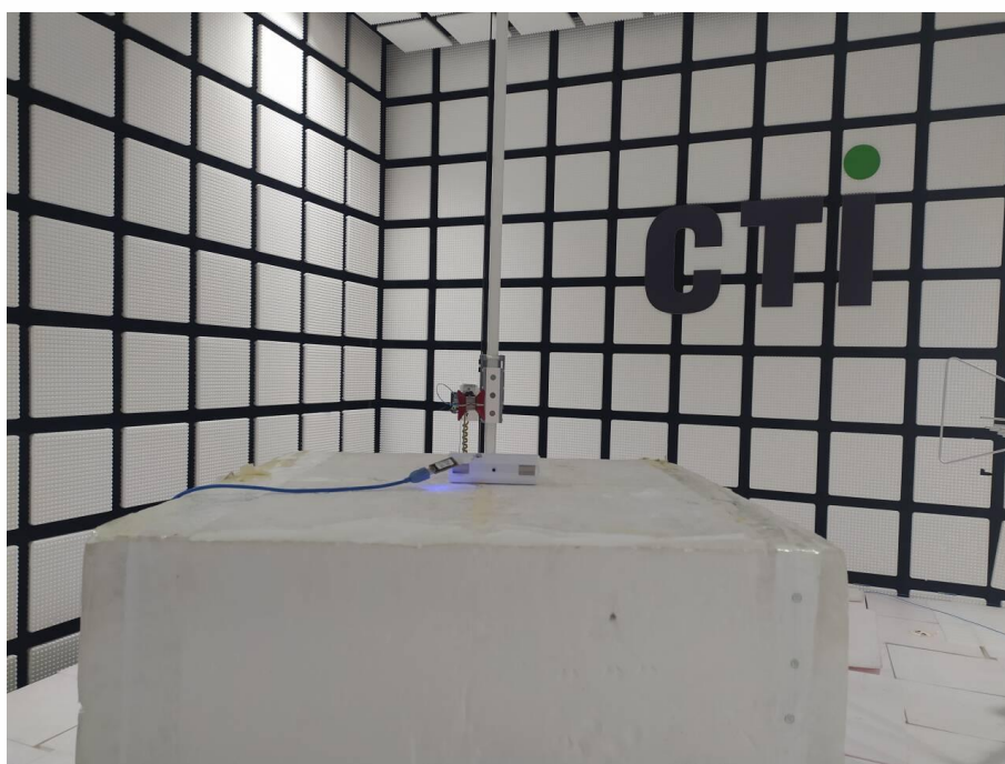
Radiated spurious emission Test Setup-2(Above 1GHz)
