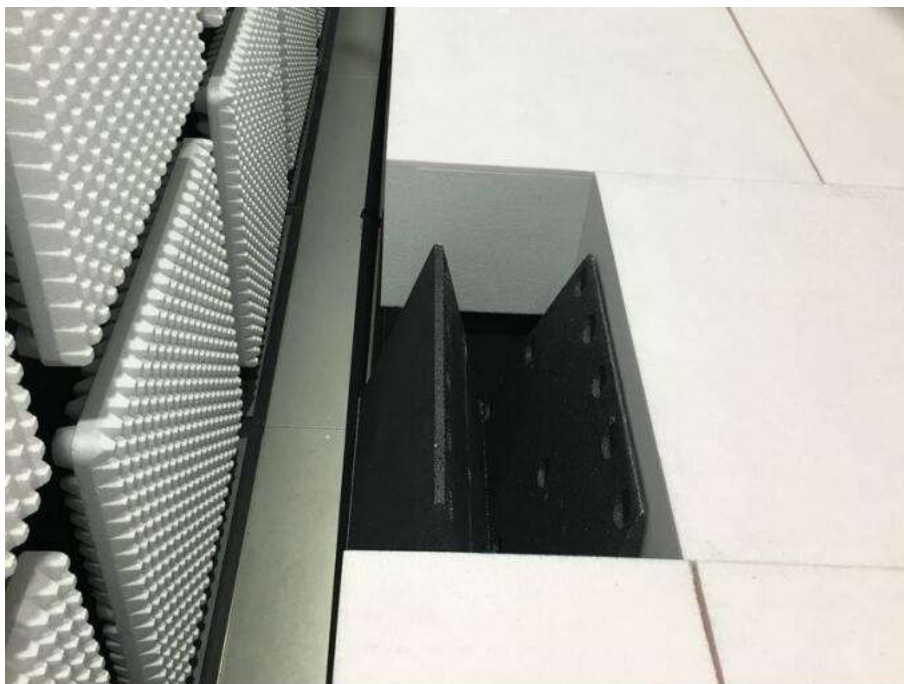
Radiated spurious emission Test Setup-2(Above 1GHz) There are absorbing materials under the ground.
