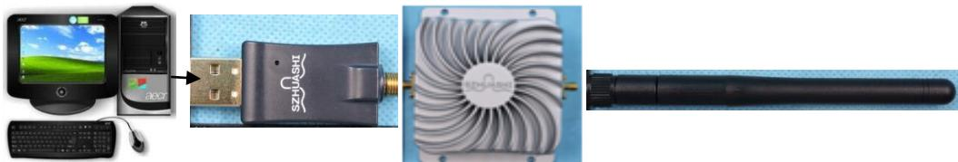
This device is a wireless USB adapter. This product adopts the specified amplifier and antenna, which will always be marketed and used as a complete system, and always be in its authorized configuration, and then input special code by professional installer to install according to the requirements of FCC regulations
