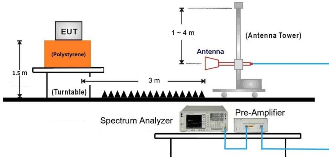
18GHz ~25GHz Test Setup:
