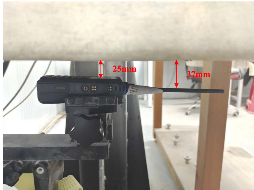
Face Up Setup Photo (25mm) (Antenna 2)
