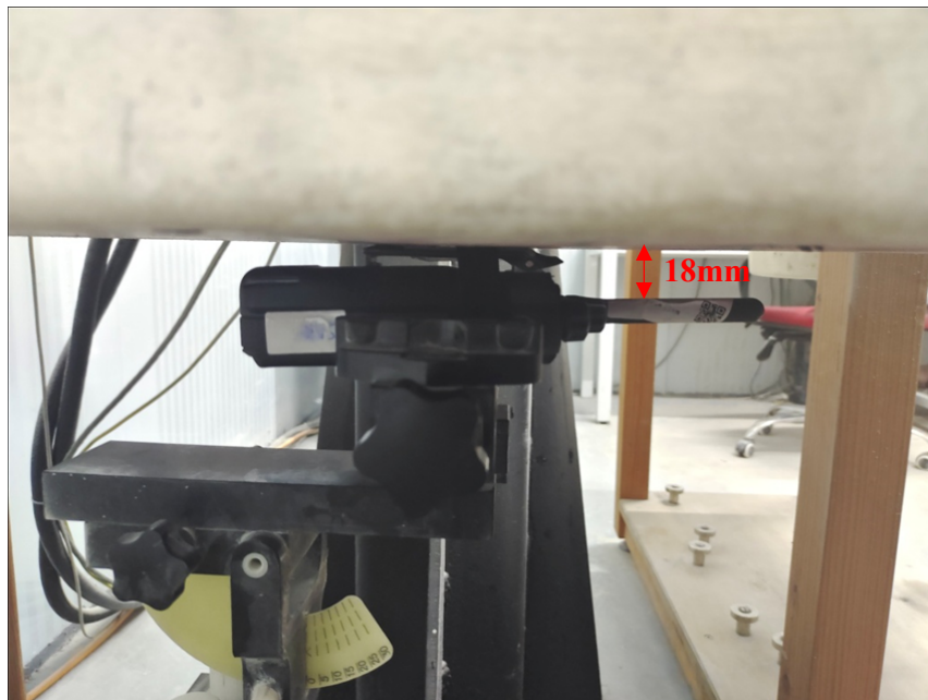
Body Back Setup Photo (0mm) (Antenna 1)
