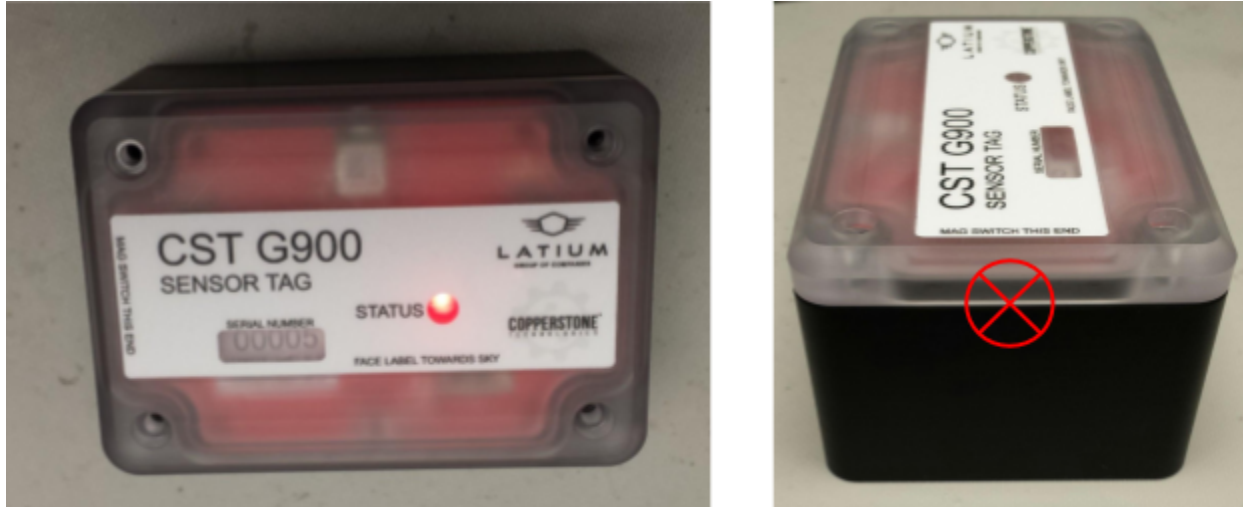
Figure 2: Serial number, status indicator, and switch location. Place magnet at marked location to activate switch.
