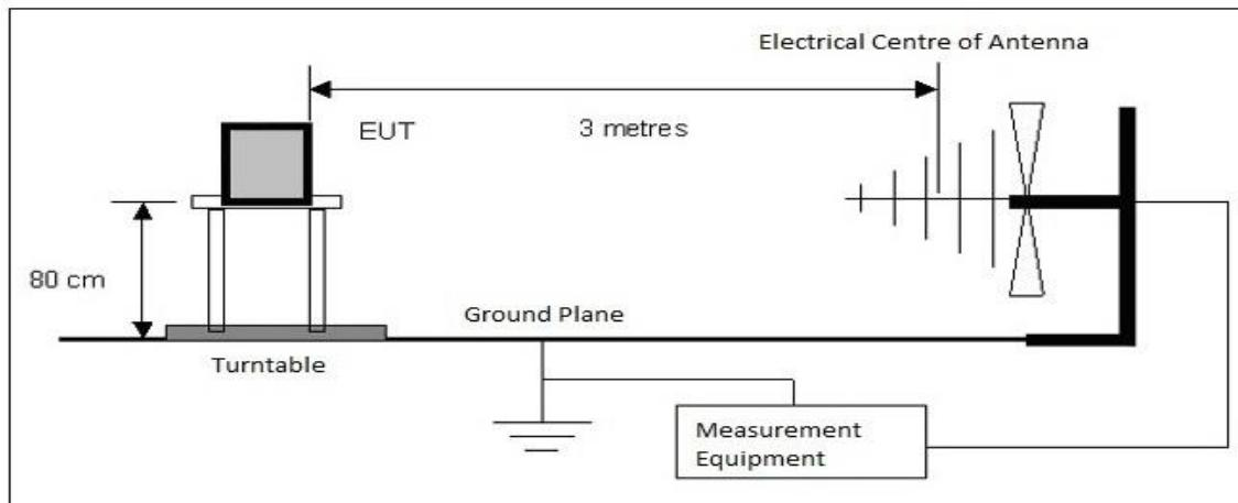
Above 1GHz, the EUT is raised using a low permittivity material (polystyrene) to a height of 1.5m.
