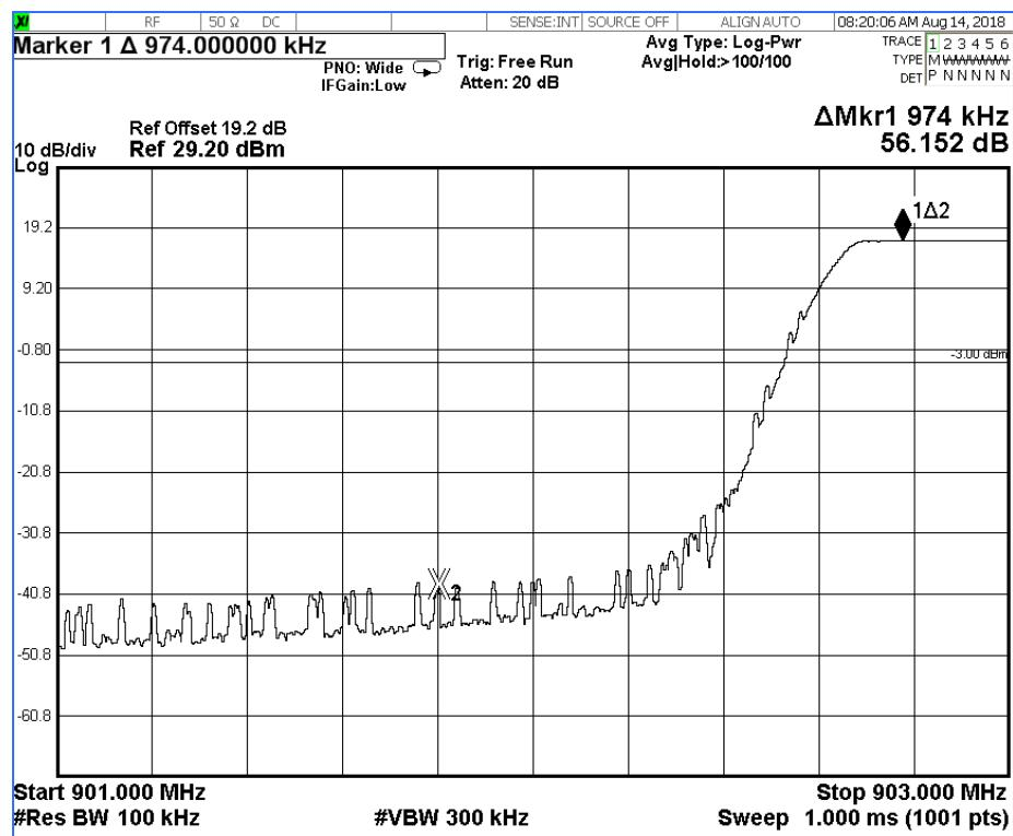
Screen Capture from the spectrum analyzer: Upper Band Edge (500 KHz DTS Mode)
