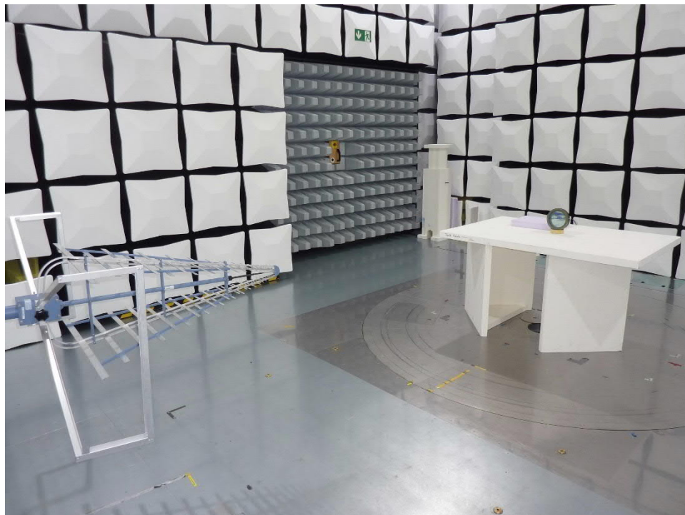
212050_08: Test setup 30 MHz to 1000 MHz
