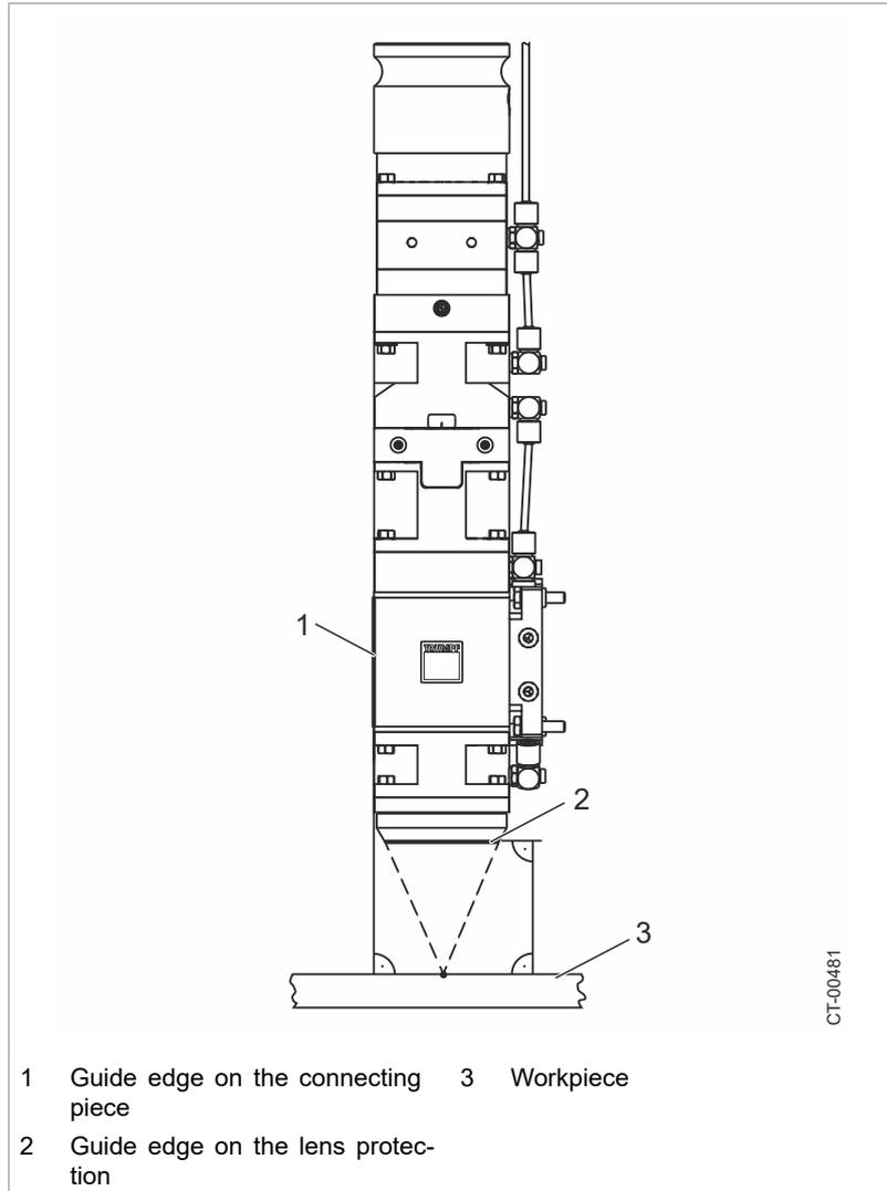
Aligning the 0° focusing optics with the processing plane
