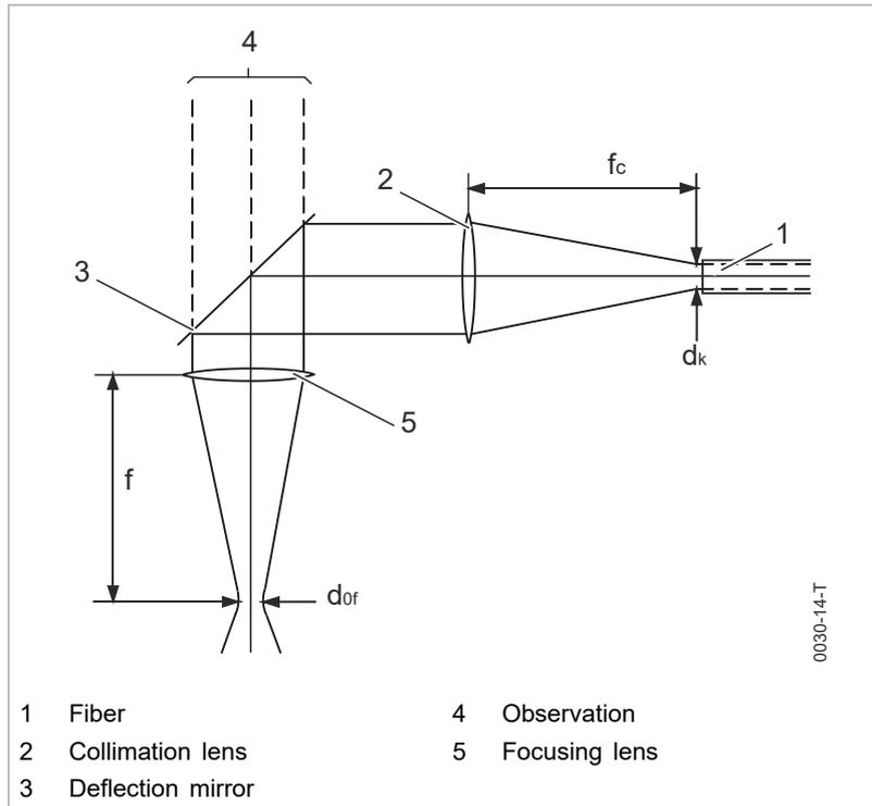
Beam guideway in a 90° focusing optics
