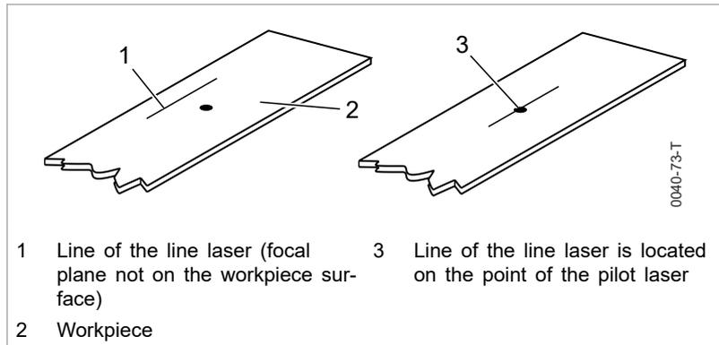
Light of the pilot laser and the line laser
