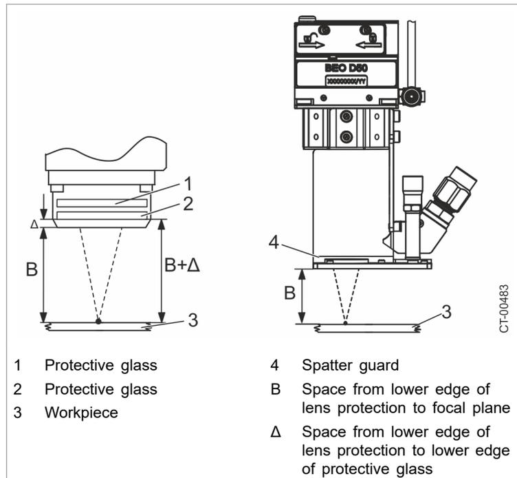
Working distance of a welding optics
