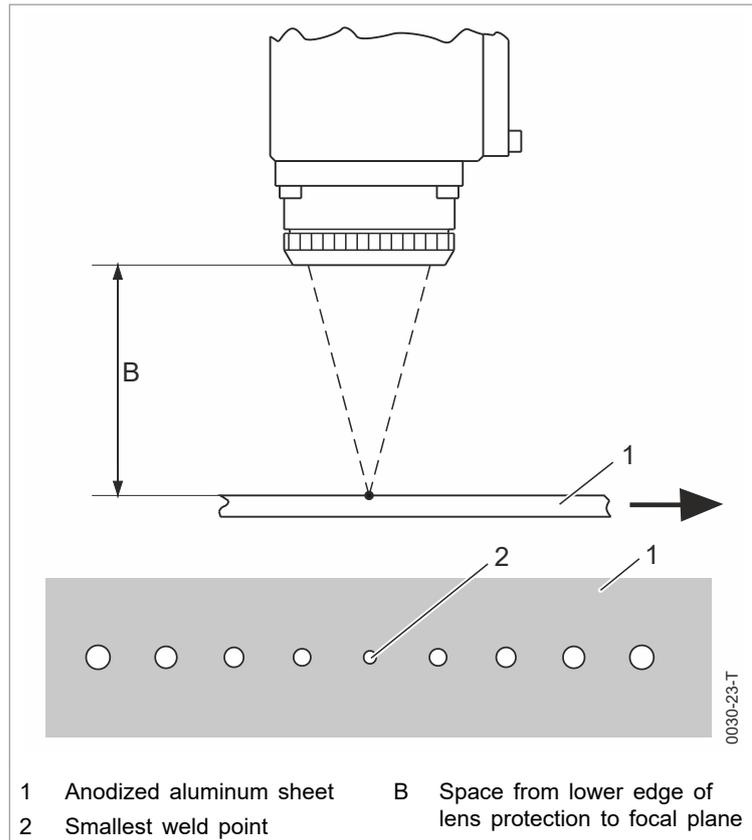
Determining the focal position with the working laser Fig. 4-5
