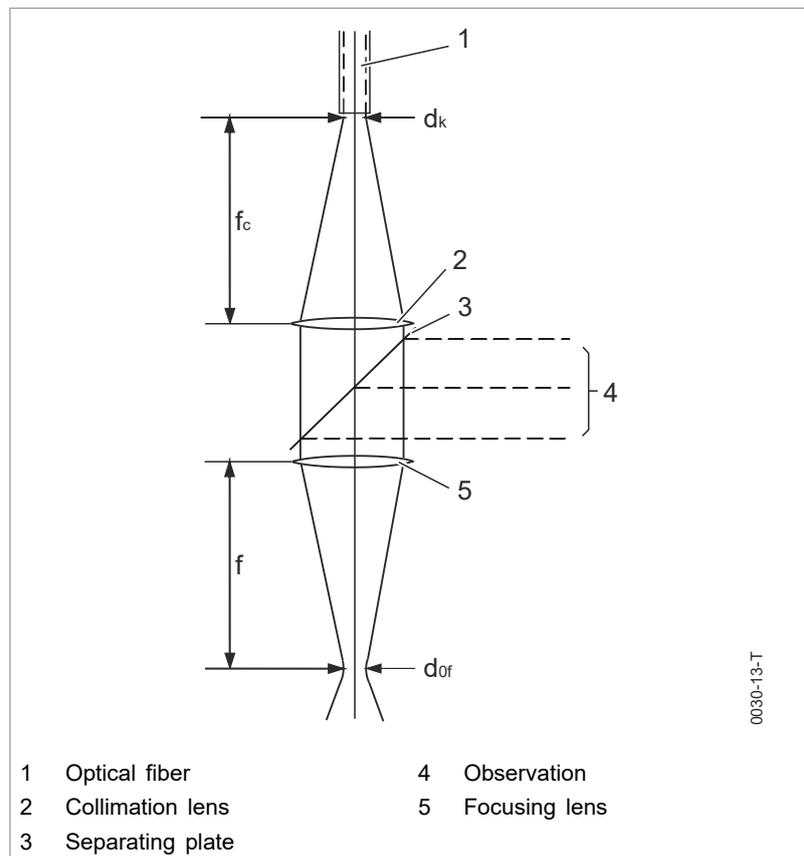
Beam guideway in a 0° focusing optics
