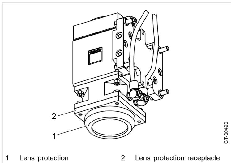
Removing the lens protection
