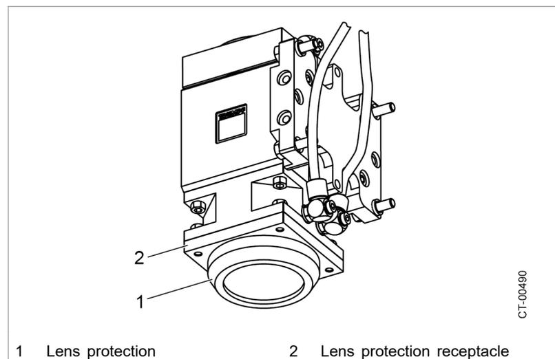
Removing the lens protection
