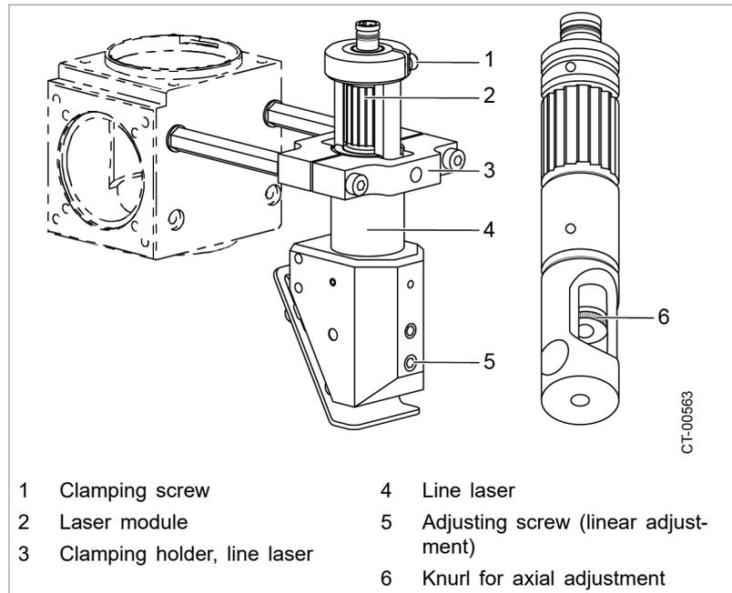
Line laser and removed laser module
