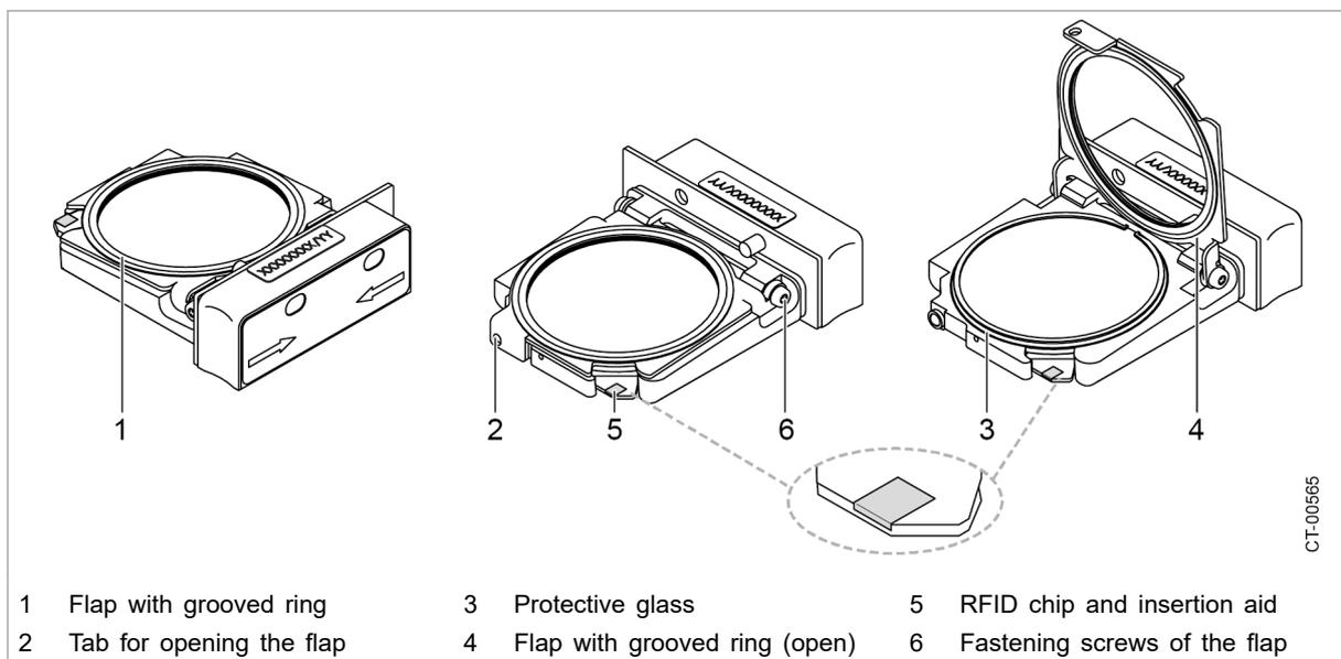
Replacing the protective glass of the objective protective glass cassette (BEO D50 Smart)
