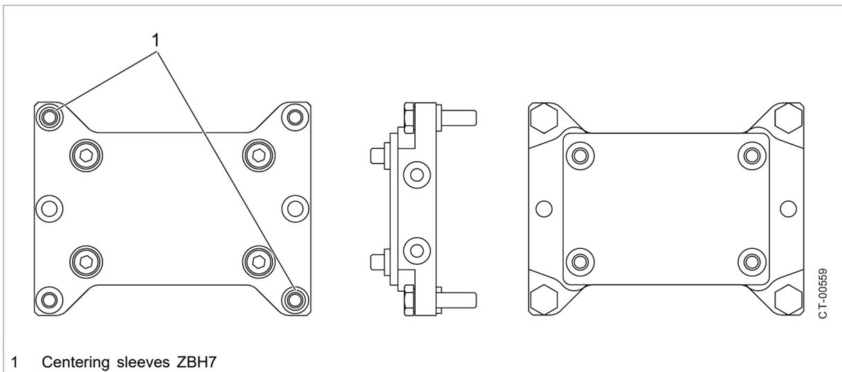
Fastening plate D50 - D70 with insulating plate
