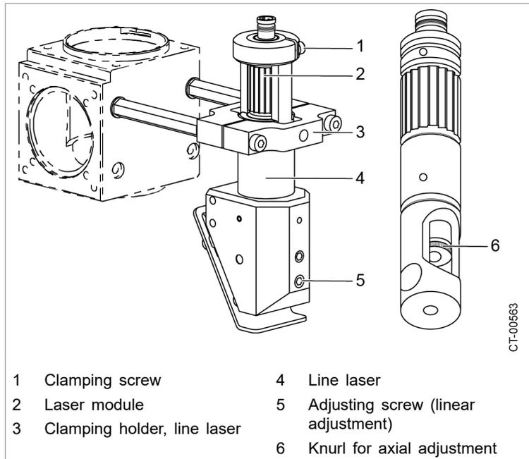
Line laser and removed laser module
