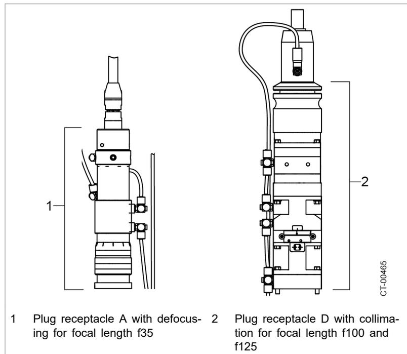
Plug receptacle A (left) and plug receptacle D (right)
