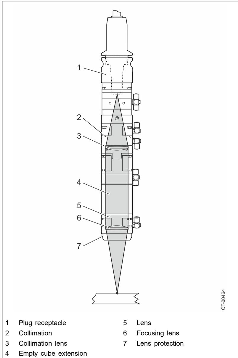
Minimum configuration of a focusing optics D50 with drawn-in beam path
