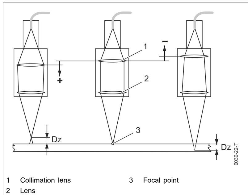
Effect of the collimation lens on the focal position
