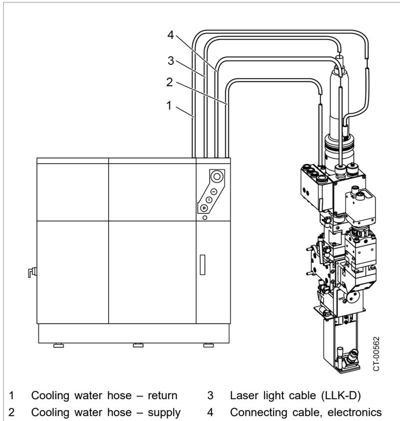
Focusing optics BEO D50 Smart, connected to a laser device (diagram) Fig. 3-43
