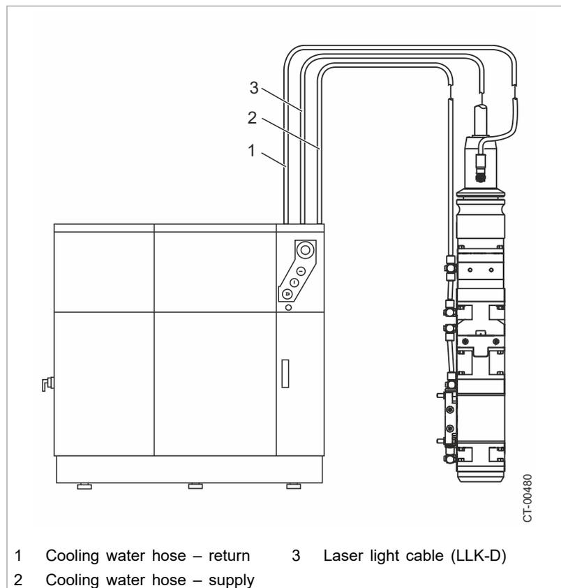
Focusing optics BEO D50 Basic, connected to a laser device (diagram)
