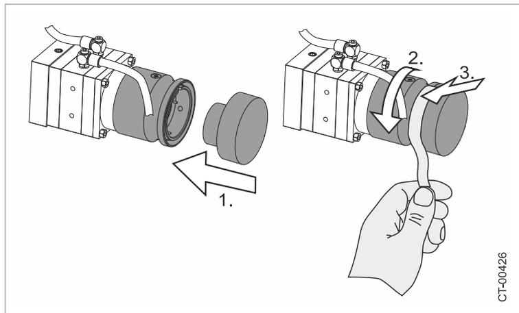
Mounting the sealing plug
