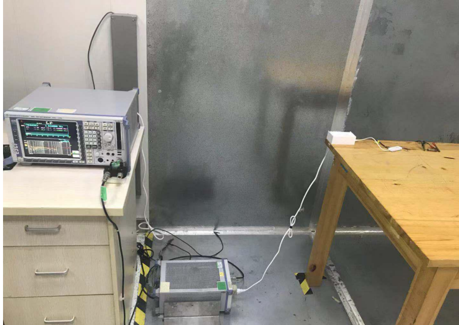
Radiated Spurious Emissions Test Frequency From 30MHz-1000MHz
