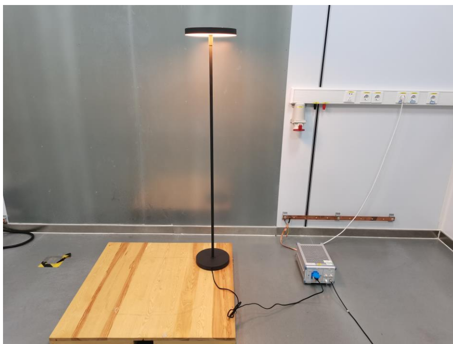
Fig. 4 Power line conducted emission setup photo
