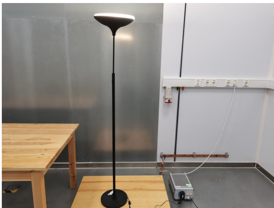
Fig. 4 Power line conducted emission setup photo
