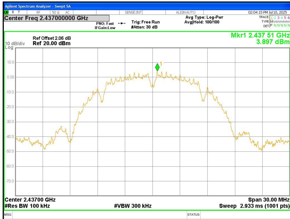
Tx. Spurious NVNT b 2437MHz Ant1 Emission
