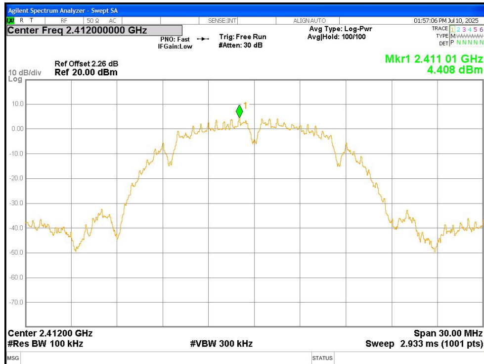
Band Edge NVNT b 2412MHz Ant1 Emission
