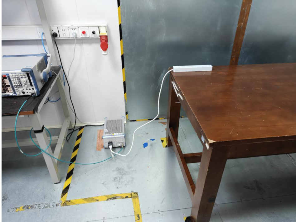
Conducted Emissions at Mains Terminals (150kHz-30MHz)
