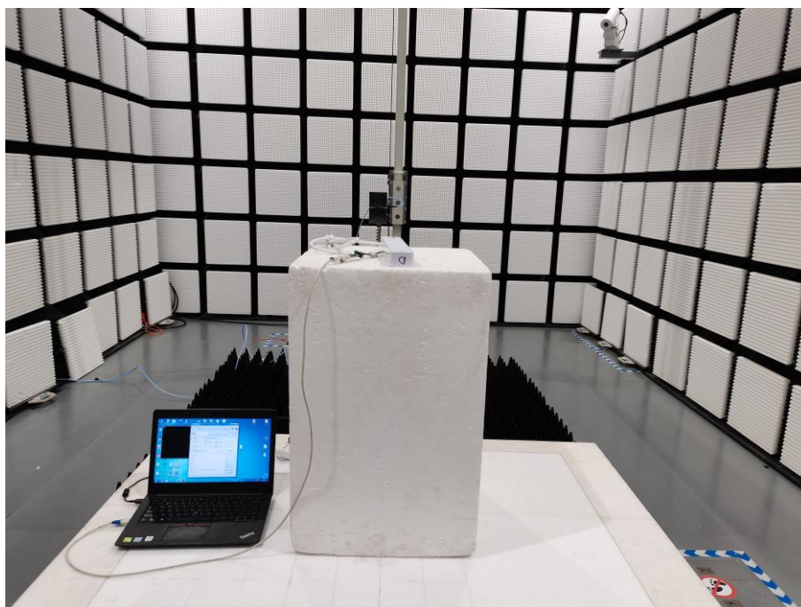
Fig. 3 Radiated emission setup photo(Above 1GHz)
