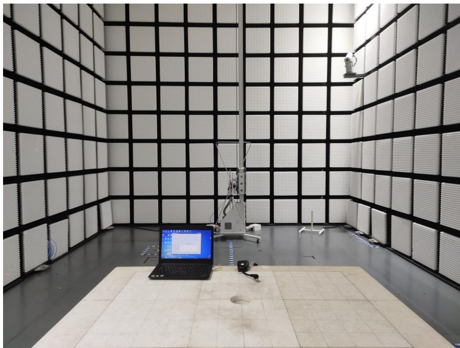
Fig. 1 Radiated emission setup photo(30MHz-1GHz)
