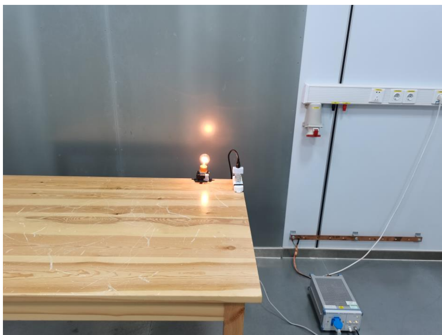
Fig. 4 Power line conducted emission setup photo
