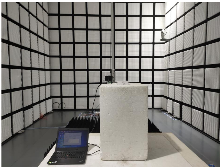
Fig. 3 Radiated emission setup photo(Above 1GHz)
