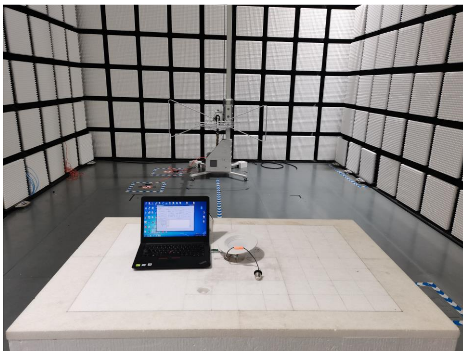
Fig. 2 Radiated emission setup photo(30MHz-1GHz)
