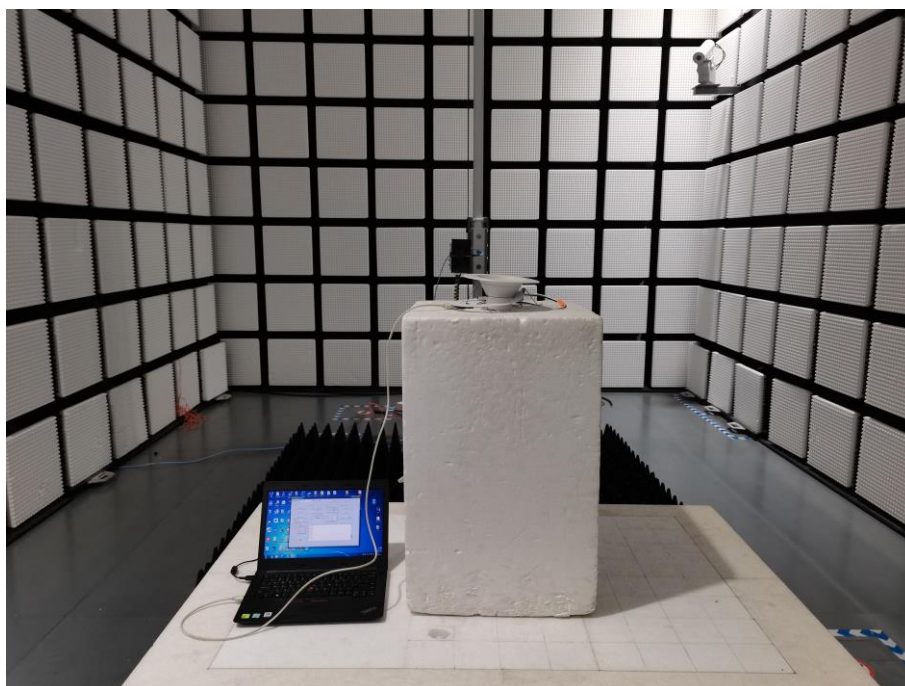
Fig. 3 Radiated emission setup photo(Above 1GHz)
