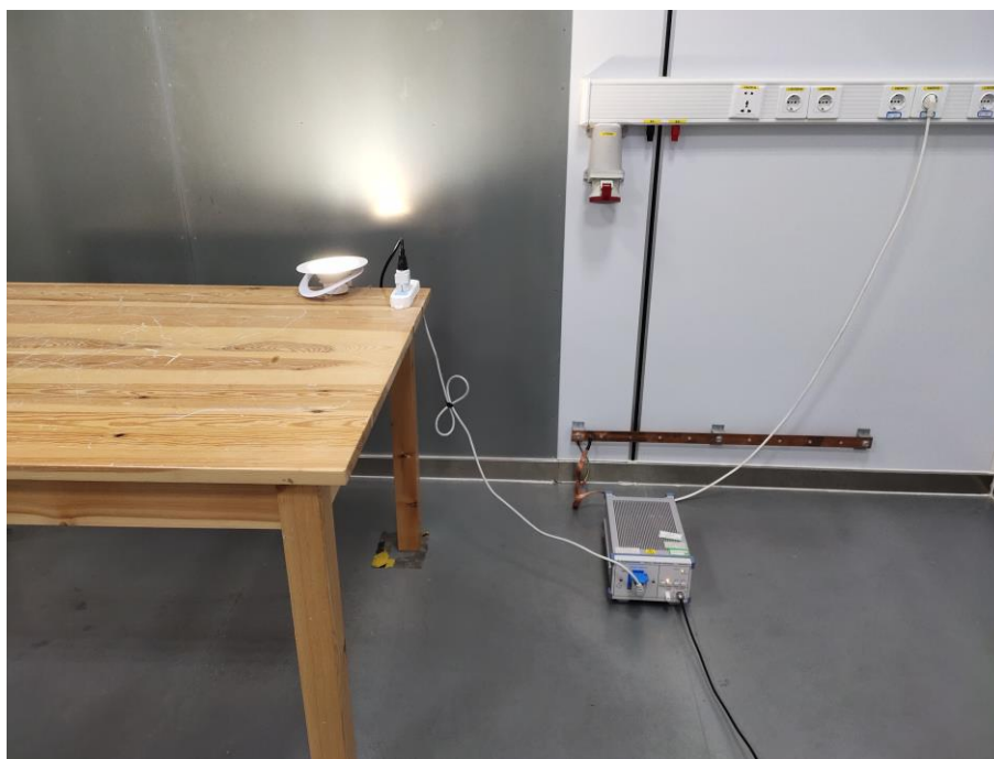
Fig. 4 Power line conducted emission setup photo
