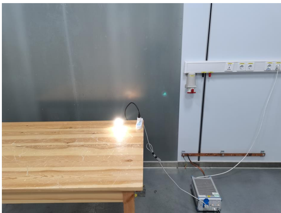
Fig. 4 Power line conducted emission setup photo
