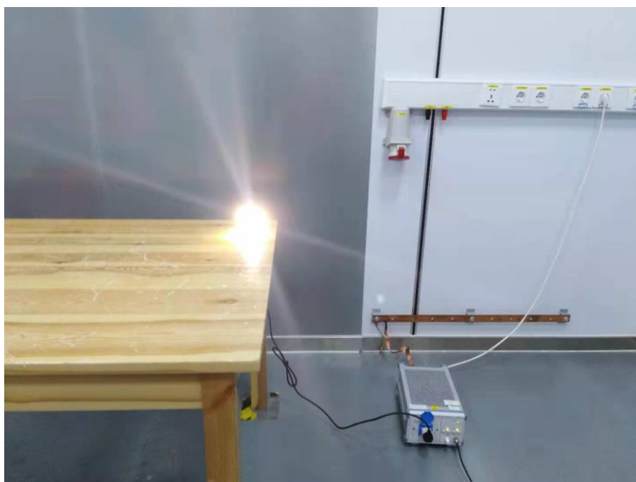
Fig. 4 Power line conducted emission setup photo
