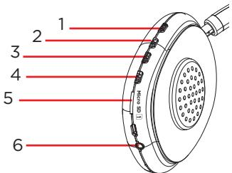
1. **Power/Mode:** Press and hold the button for three seconds to turn the headphones On and Off. Press the button to change the mode.
