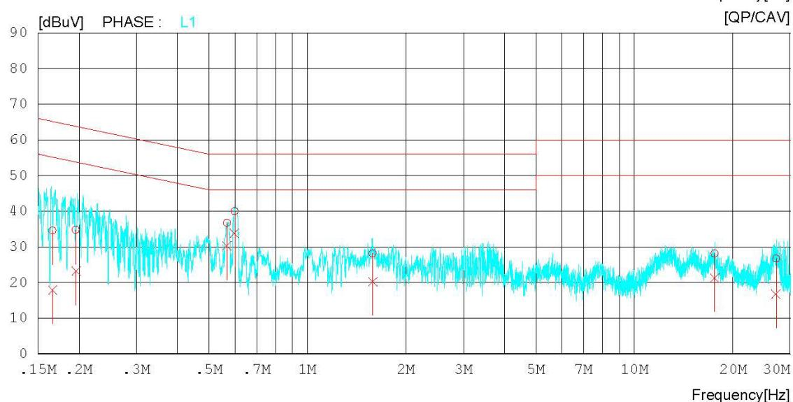
**Measurement Data (5W)****Results of Conducted Emission**
