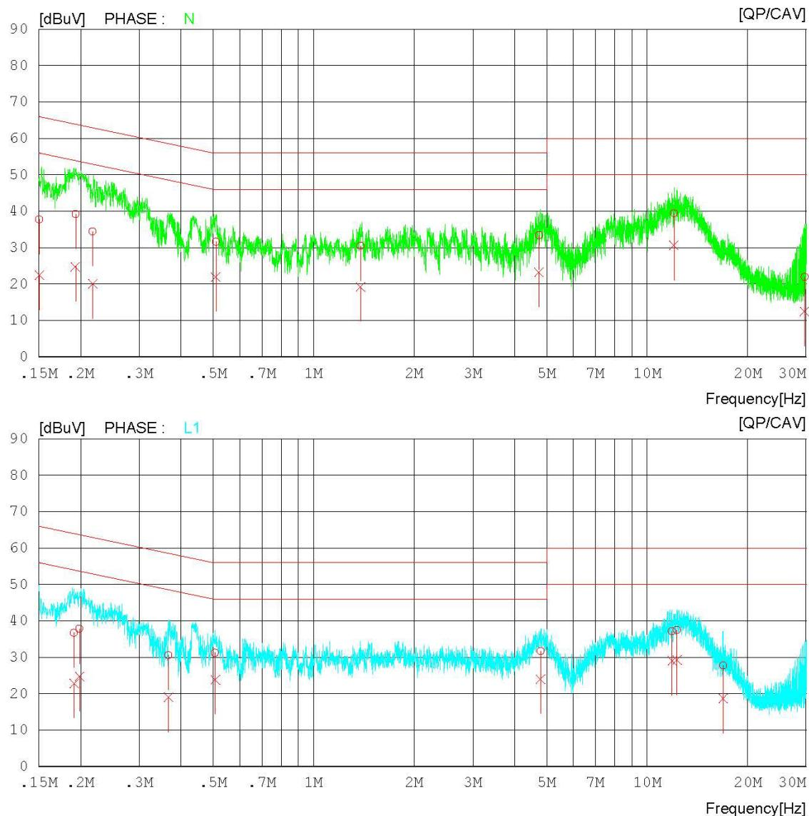
**Measurement Data (5W)****Results of Conducted Emission**
