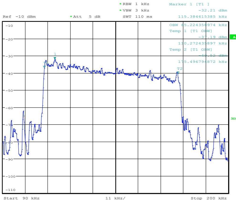
According the test data above, the fundamental wave is not fall in the restricted band 90KHz-110KHz, the field strength also meet the 15.209 requirement, please refer to clause 7.3.
