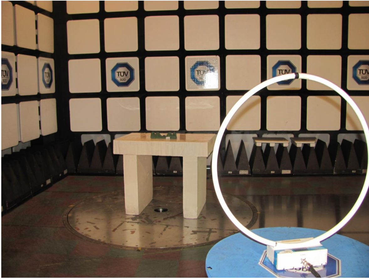
Figure 1 – Radiated Emissions Setup – Photo 1
