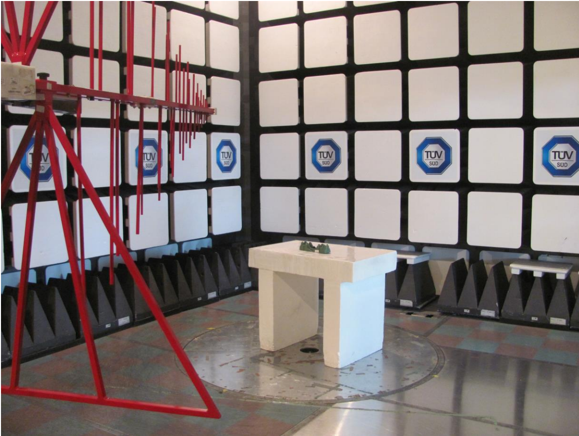
Figure 2 – Radiated Emissions Setup – Photo 2
