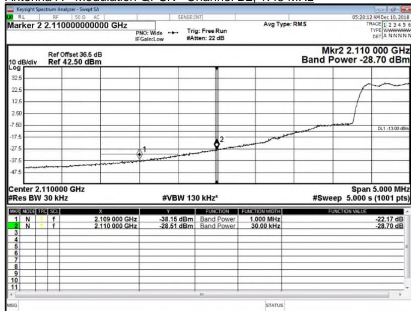
Antenna A - Modulation QPSK - Channel T2, 1.48 MHz
