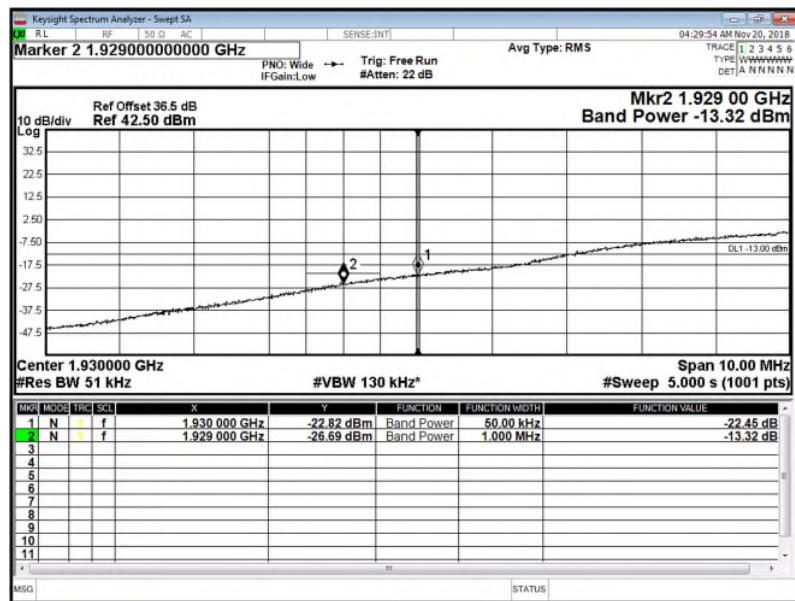
Antenna A - UMTS Modulation QPSK - Channel T2, 5MHz
