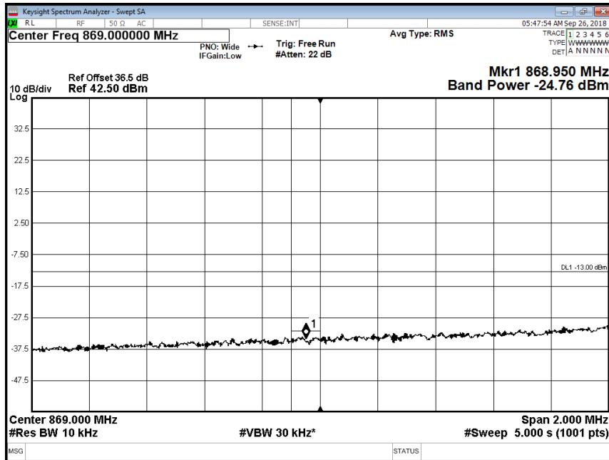
Antenna A - LTE Modulation QPSK - Channel T2, 5MHz
