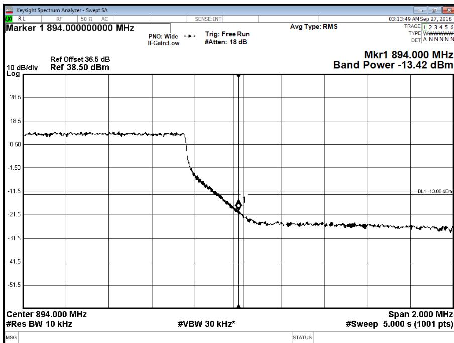
Maximum Target Output Power T2:43dBm B2:43dBm
