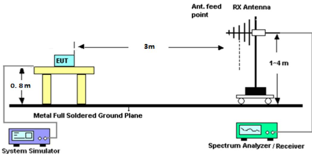
For radiated test from above 1GHz
