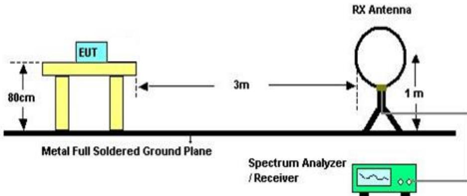
The setting of the spectrum analyzer
