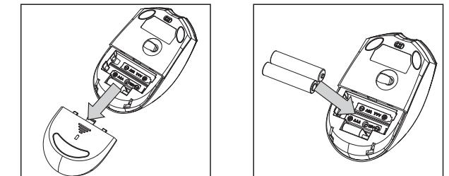
1. Open the battery cover on the bottom of the mouse.
