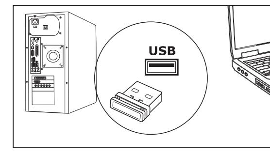
2. Insert a nano receiver into spare USB port.
