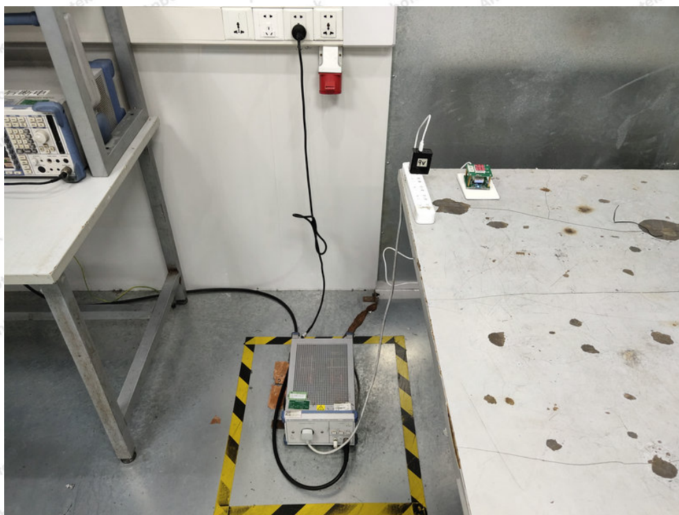
Photo of Conducted Emission Measurement
