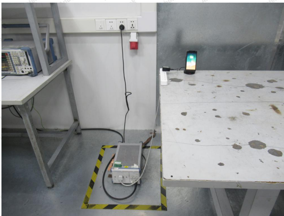
Photo of Conducted Emission Measurement
