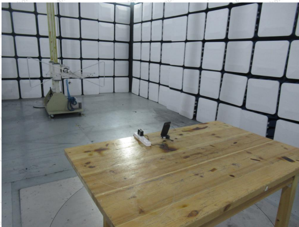
Photo of Radiation Emission Test
