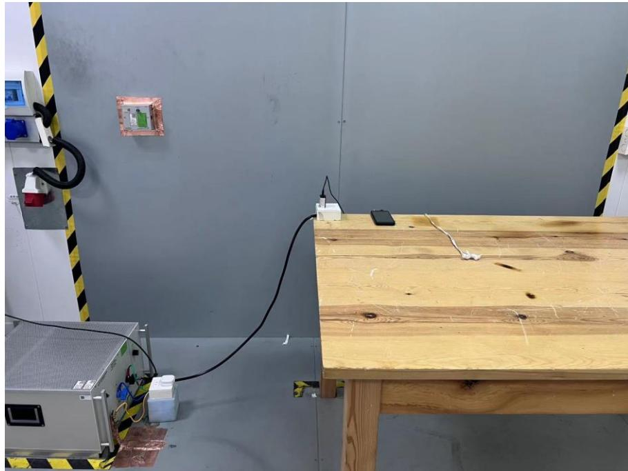
**Set-up for Radiated Emission (RE), Below 1GHz**
