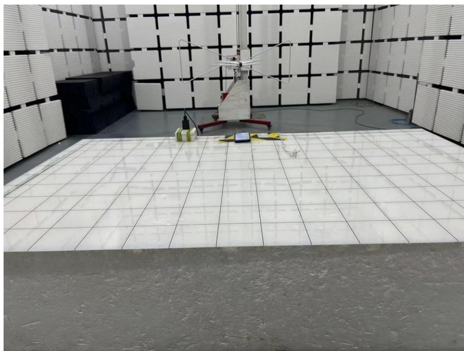
**Set-up for Radiated Emission (RE), Above 1GHz**
