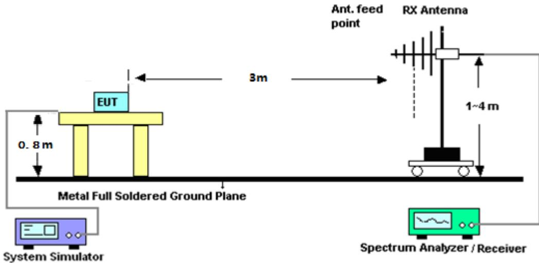
For radiated test from above 1GHz
