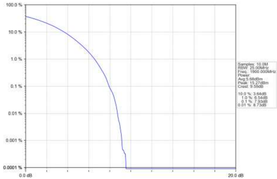
n2_30kHz_SISO_NTNV_20MHz_CP-OFDM 64 QAM 1900MHz_Outer_Full_Ant1
