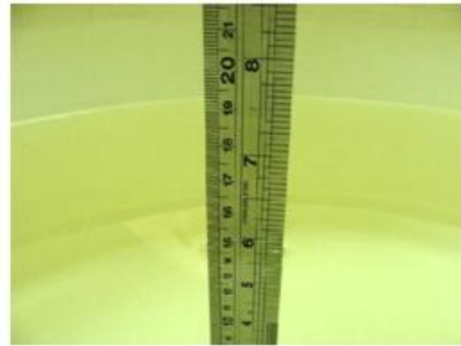
Fig 7.2 Photo of Liquid Height for Body SAR
