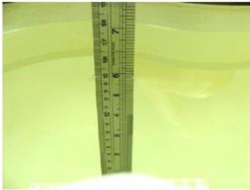
Fig 7.1 Photo of Liquid Height for Head SAR
