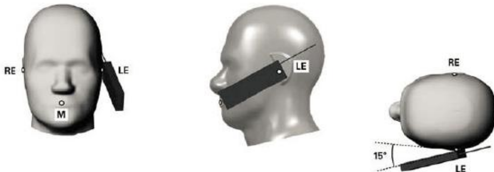
Fig.9.4 Illustration for Tilted Position
