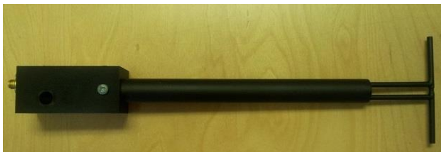
Figure 1 – MVG COMOSAR Validation Dipole
